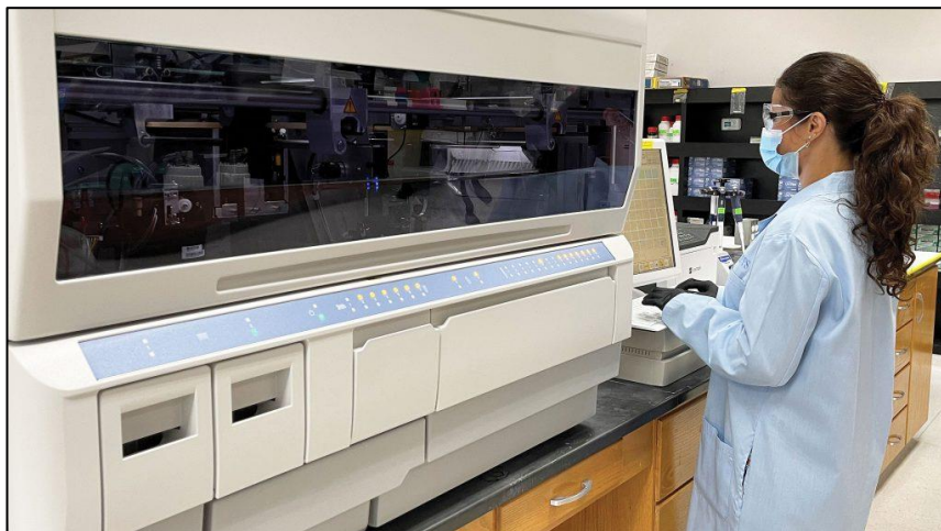
Successful recombinant protein development requires extensive testing using antibody-based assay systems. Shown here is a Scripps Laboratories scientist evaluating recombinant apoferritin on a high-throughput clinical immunoanalyzer. Thorough testing is essential for producing recombinant proteins that will perform comparably to their native counterparts in a clinical diagnostic setting.
