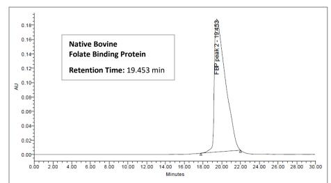
**Figure 2.** HPLC profile of native bovine Folate Binding Protein. Analysis was performed using a Biozen 3  $\mu$ m dSEC-2, 200 Å, 300 x 7.8 mm column.
